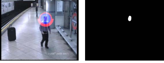
Figure 4. Left: input video frame with localized search region indicated by red circle. Right: the Cr detection result within the search region. AVSS 2007 video dataset.
